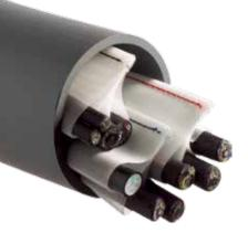
OptiCell™ innerduct is a flexible fabric system designed specifically for increasing conduit capacity. The unique textile construction allows OptiCell™ innerduct to conform to the shape of cables placed within, greatly reducing wasted space and increasing cable deployment efficiency.
